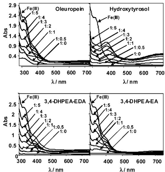
**Figure 1.** Chelate formation of phenolic compounds at  $400 \mu\text{M}$  in the presence of increasing ferric ion concentrations at pH 3.5. Fe(III) is solution of ferric chloride at  $2000 \mu\text{M}$ .
